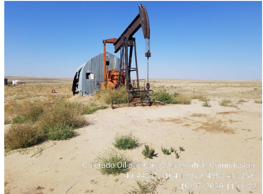
Photo 2 – Pumping Unit – Stained Soil, WEEDS, Debris, Unused Equipment
