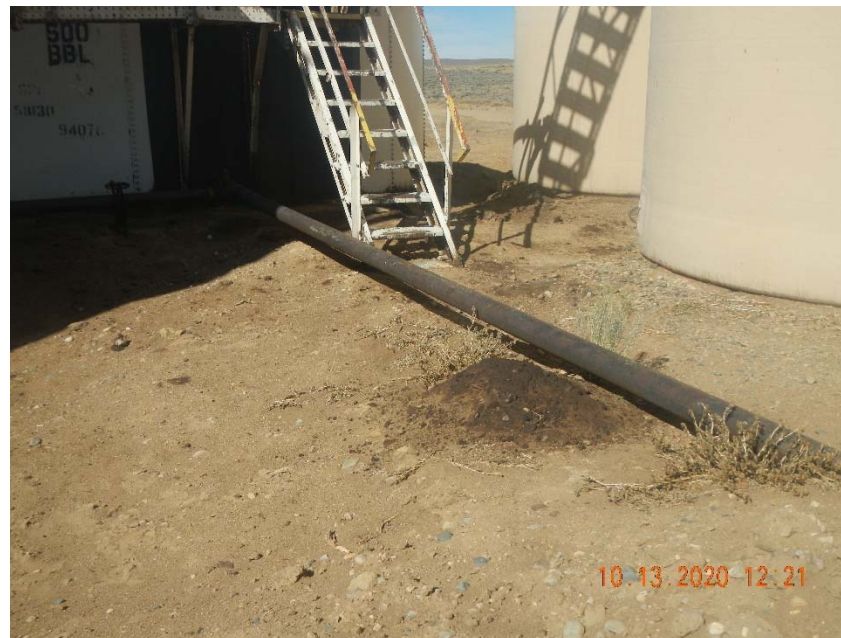
Photo 4. Example of stained soil in tank battery.
