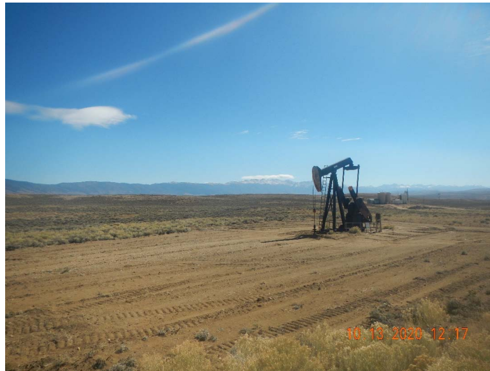
Photo 1. Overview of location facing southeast. Freshly disturbed soil with no stormwater controls.
