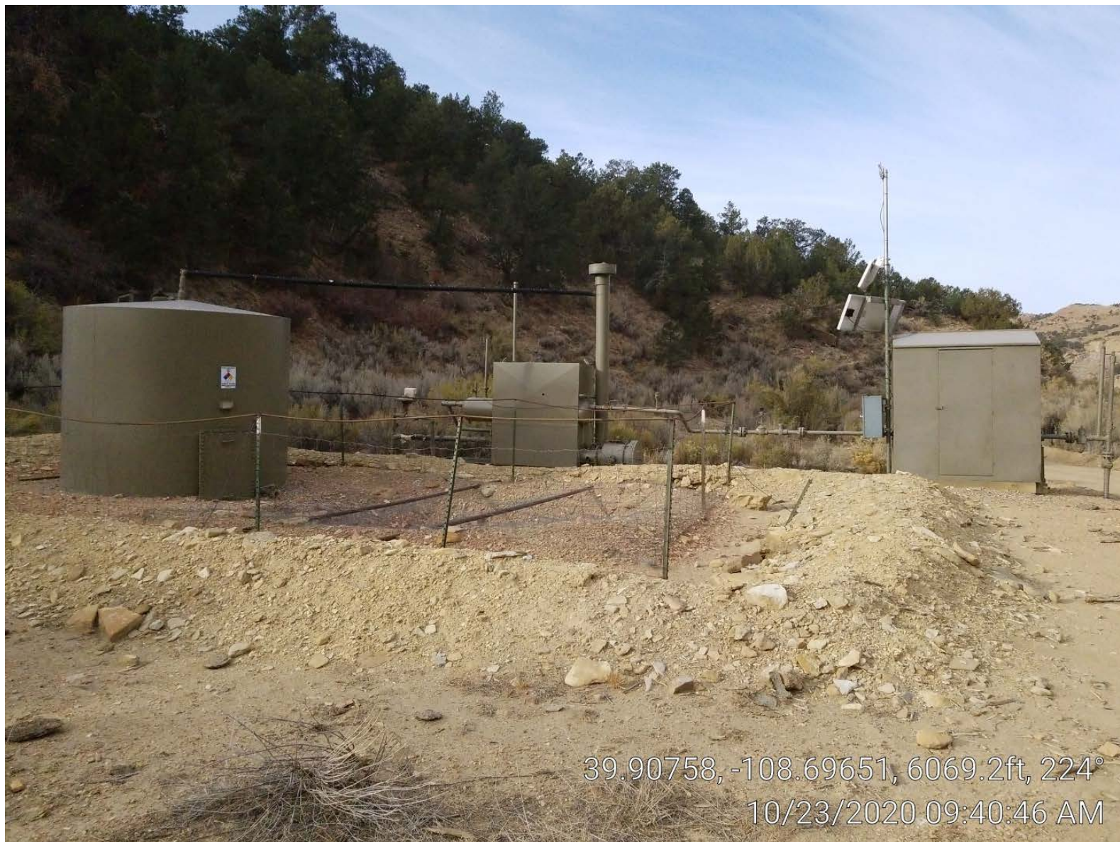
Photo 2. Tank, pit, separator, meter building.
