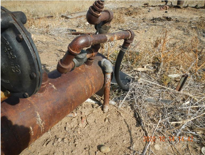
Photo 5: Gas vessel and 1' flowlines.
