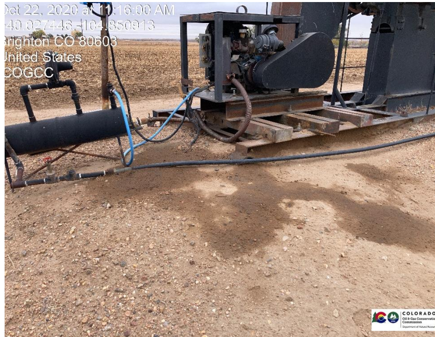
Pic 1 stained soil by pumping unit motor
