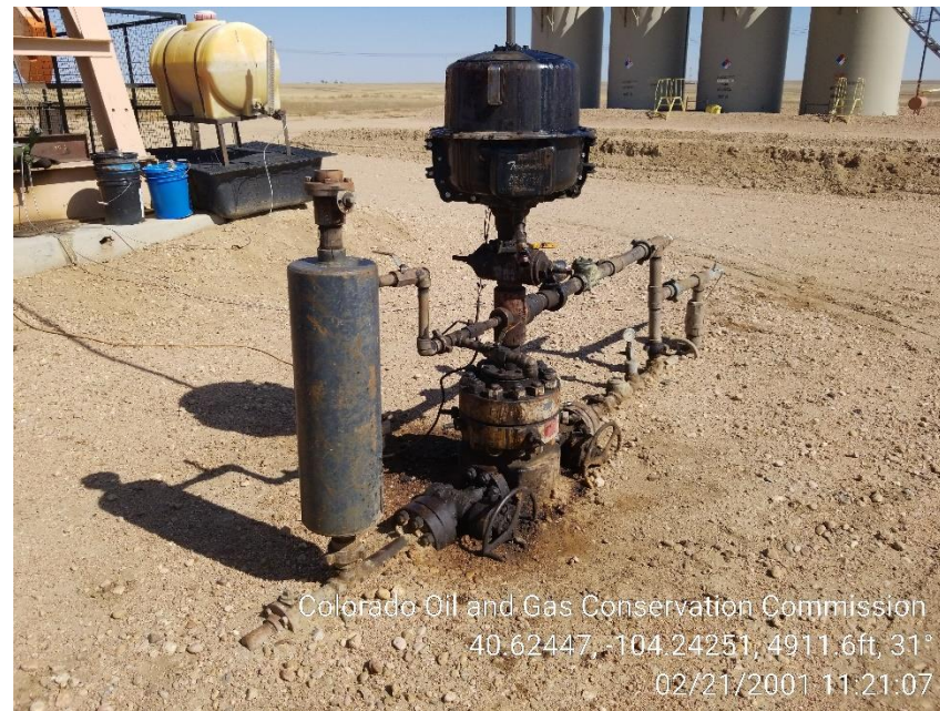
Photo 6 – Wellhead, Stained Soil
