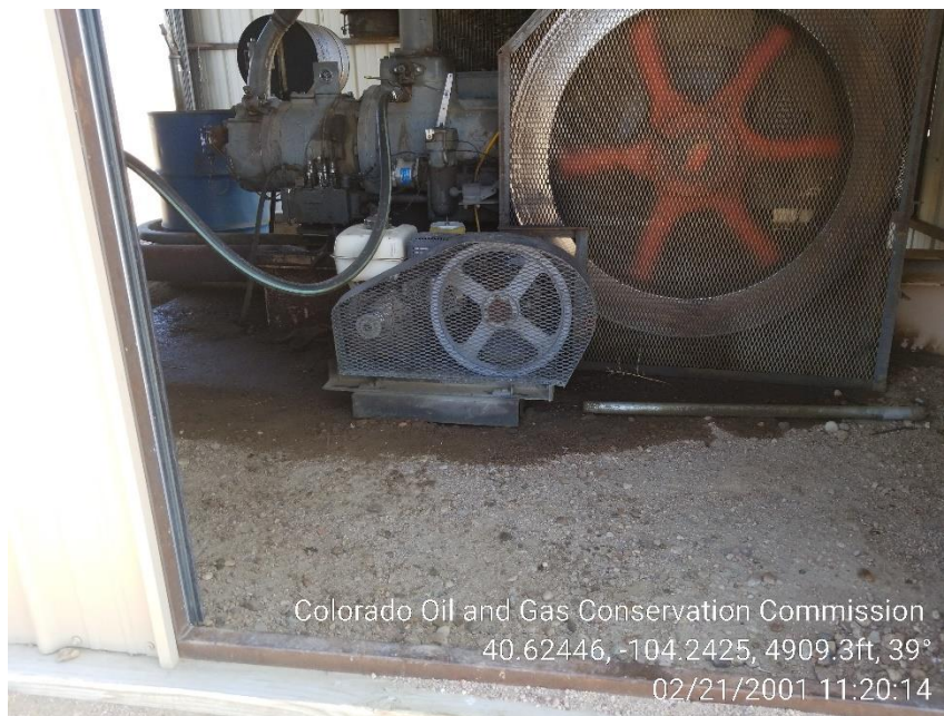
Photo 9 – Stained Soil at Gas Engine
