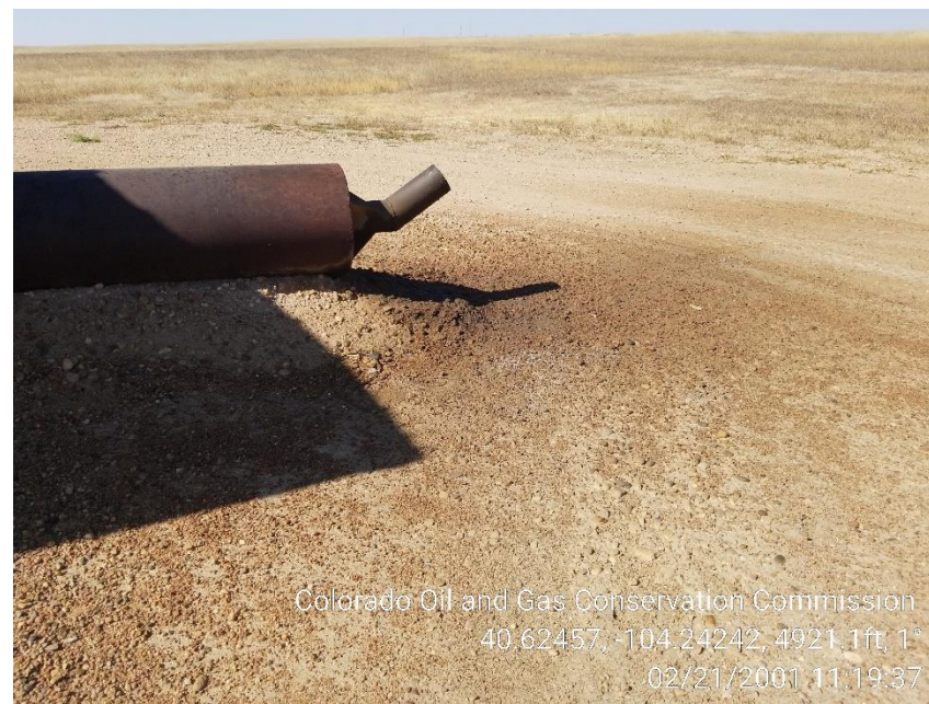
Photo 10 – Stained Soil at Exhaust
