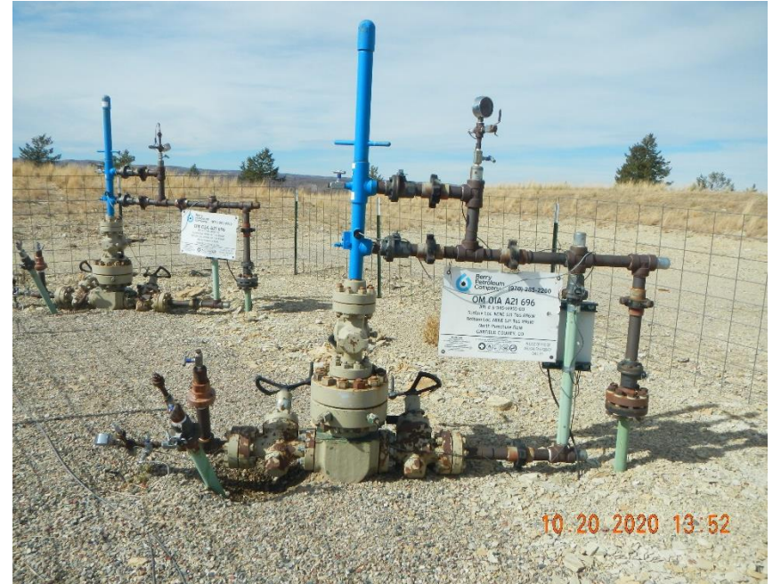
Fluid leaking from wheel valve on OM1A A21 696 annulus.
