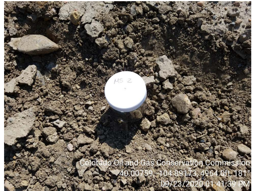
Photo 8 – Soil sample 2; taken from soil runoff area with no vegetation. Soils are very well compacted.
