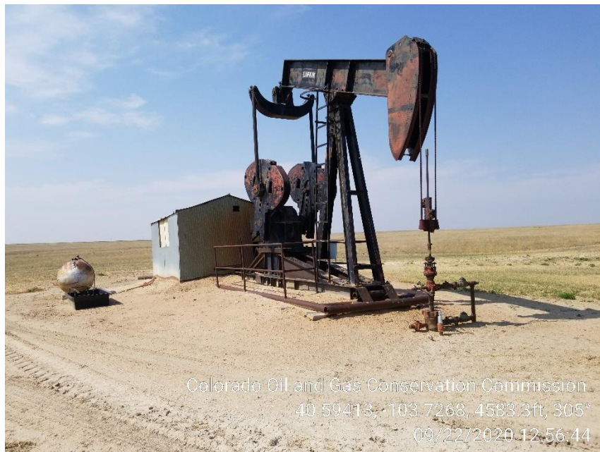
Photo 5 – Pumping Unit, weeds removed
