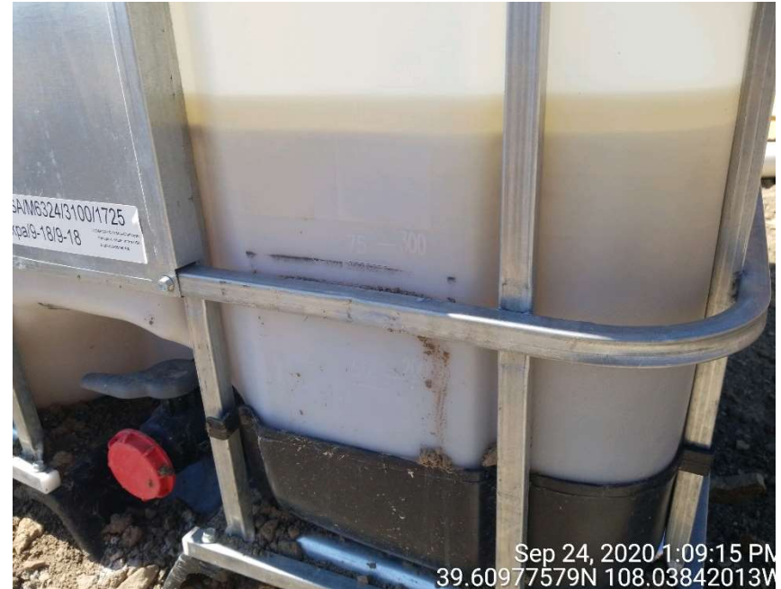
Fluid in the cube container with two distinct visible layer.
