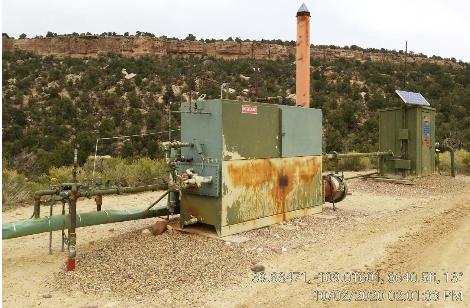
Photo 3. Separator & meter building.
