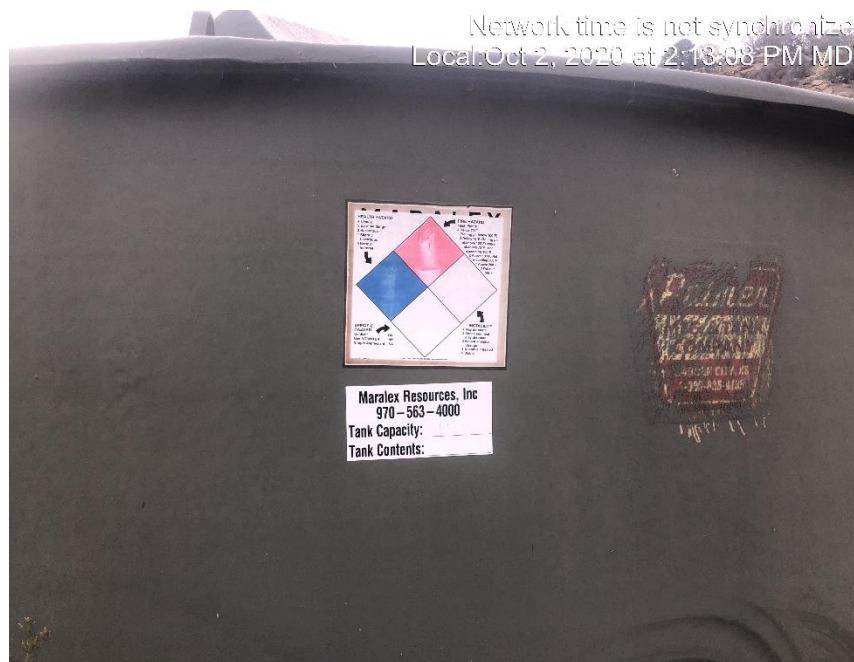
Photo #1976 Tank label weathered and not legible.
