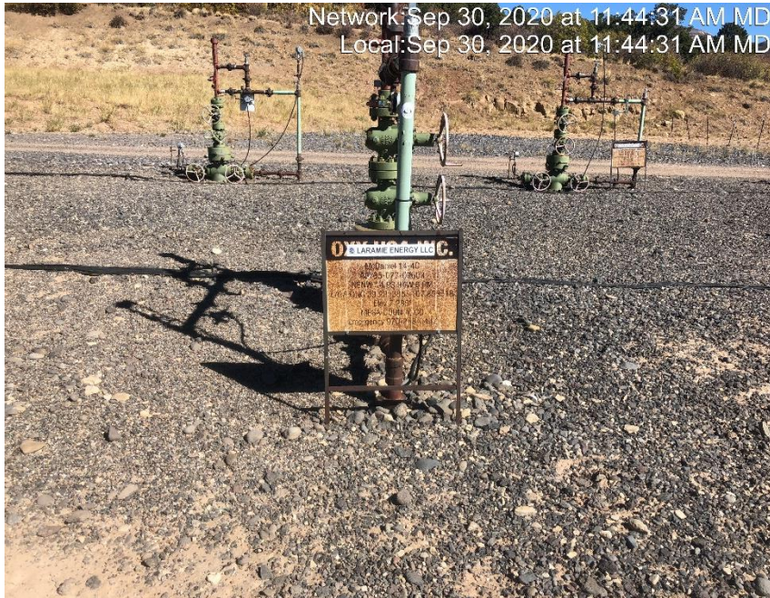
Photo #1959 Multiple wellhead signs weathered and not legible.
