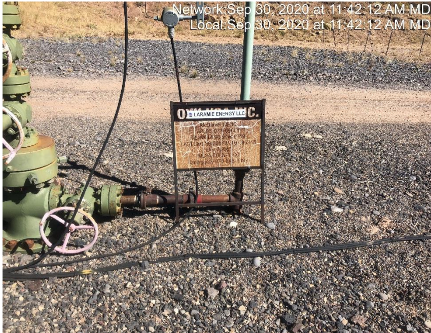
Photo #1957 Multiple wellhead signs weathered and not legible.
