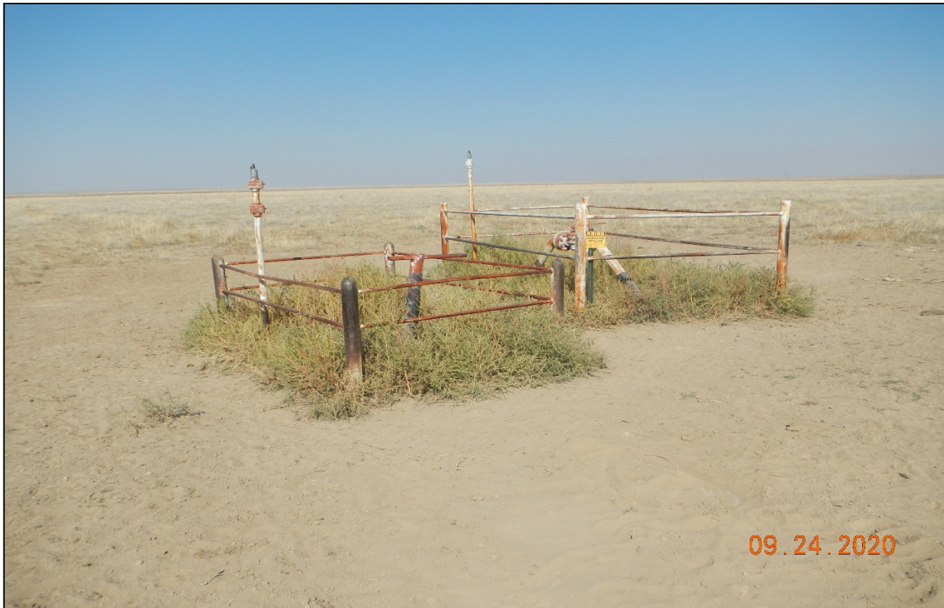
Photo 3. There is pipe risers associated with the former well site that have not been removed.
