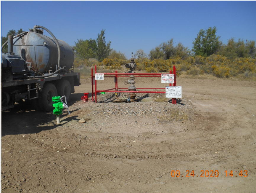
Injection wellhead. Temporarily Abandoned.
