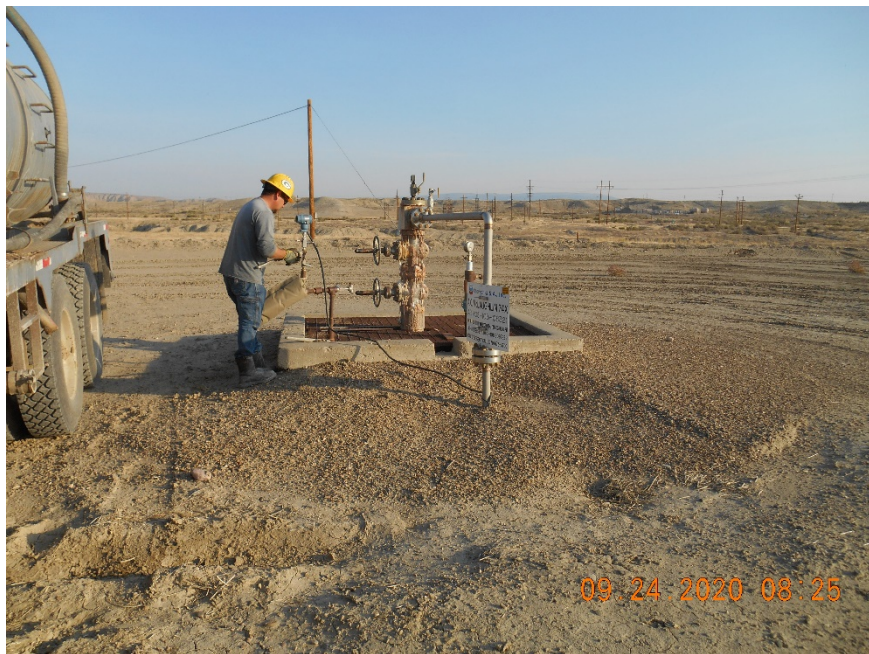
Injection wellhead.
