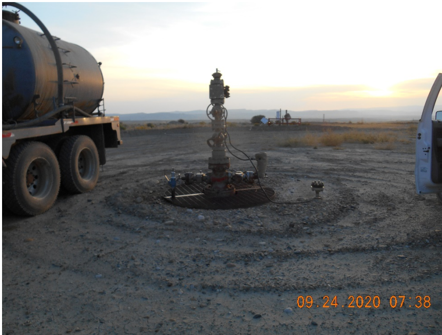
Injection wellhead
