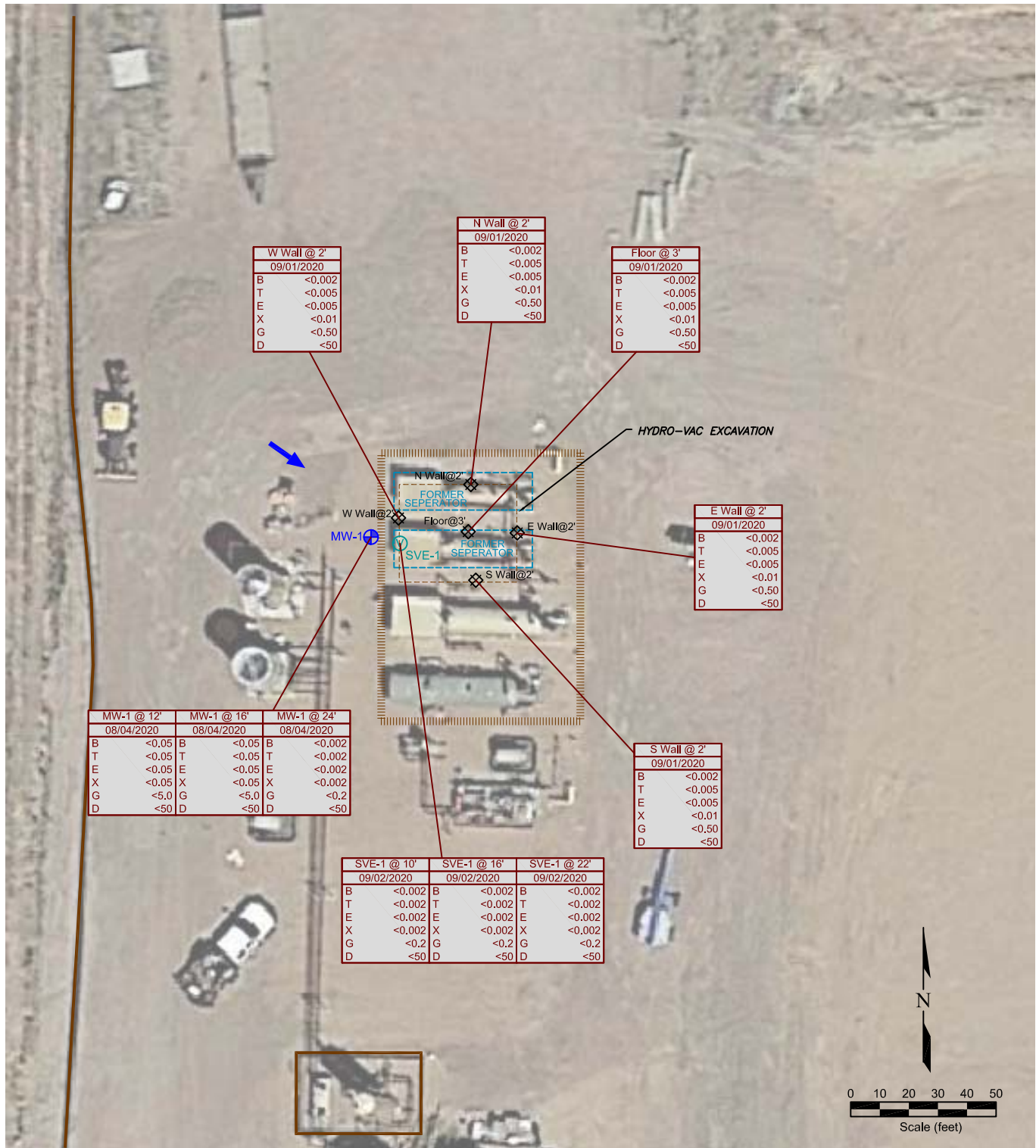
Figure 3 EXTENT OF EXCAVATION WITH SOIL CHEMISTRY MAP GREAT WESTERN OPERATING COMPANY T & M Tank Battery SWSW Sec. 15 T8N, R66W ~ 40.65564°, -104.77254° Weld County, Colorado
