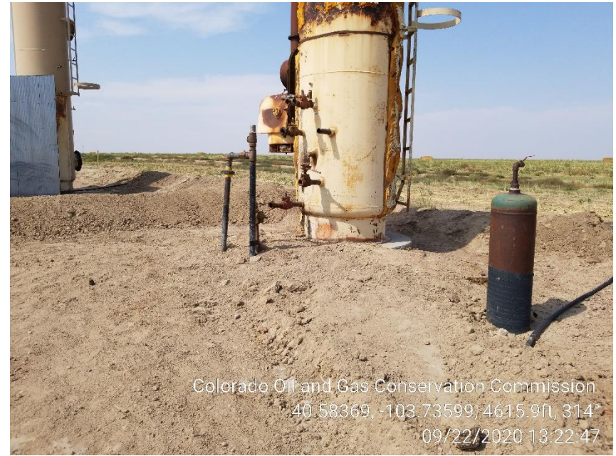
Photo 6 – East Heater Treater; disconnected no longer in use. Risers marked
