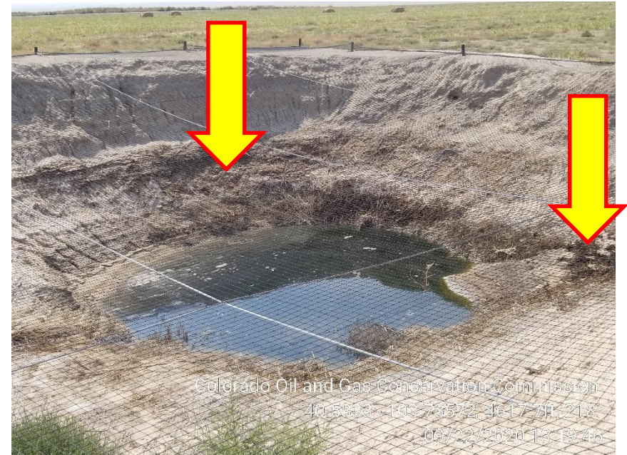
Photo 12 – Oil/Hydrocarbon on Pit. Stained Soil on the Edges
