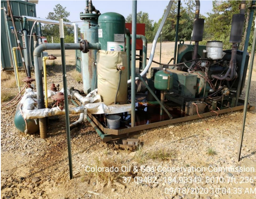
Photo 3 Stained soil at liquid ring
