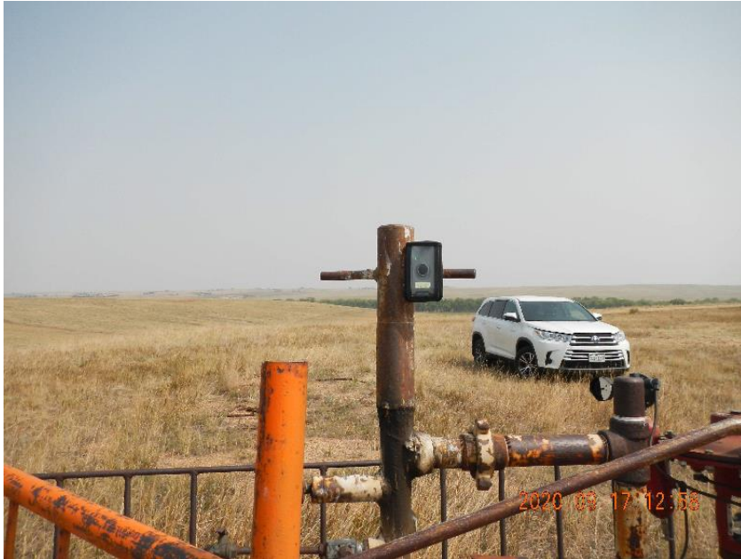
Photo 1: View of Trimble GPS unit at wellhead.
