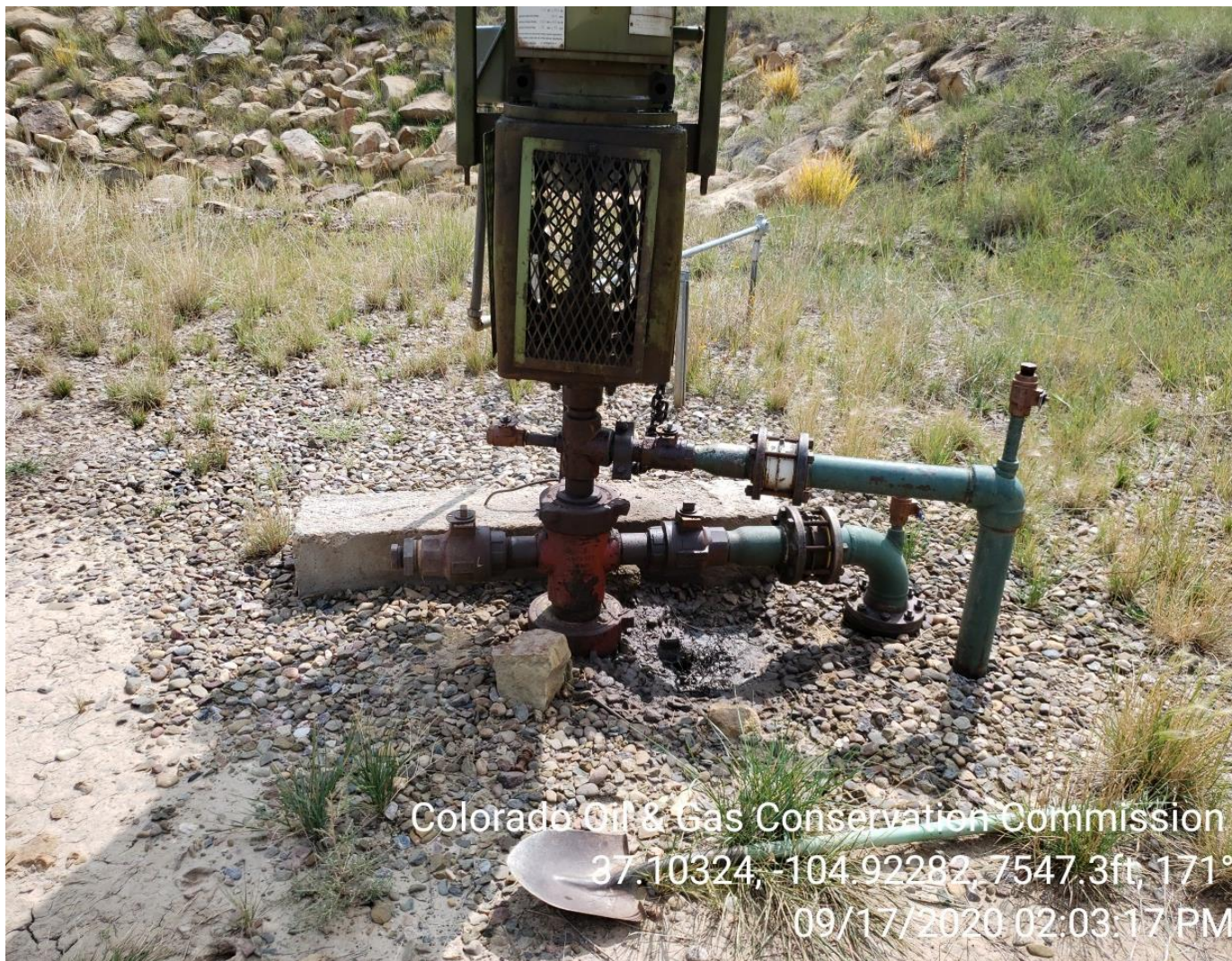
Photo 5: Stained soil at drive head
