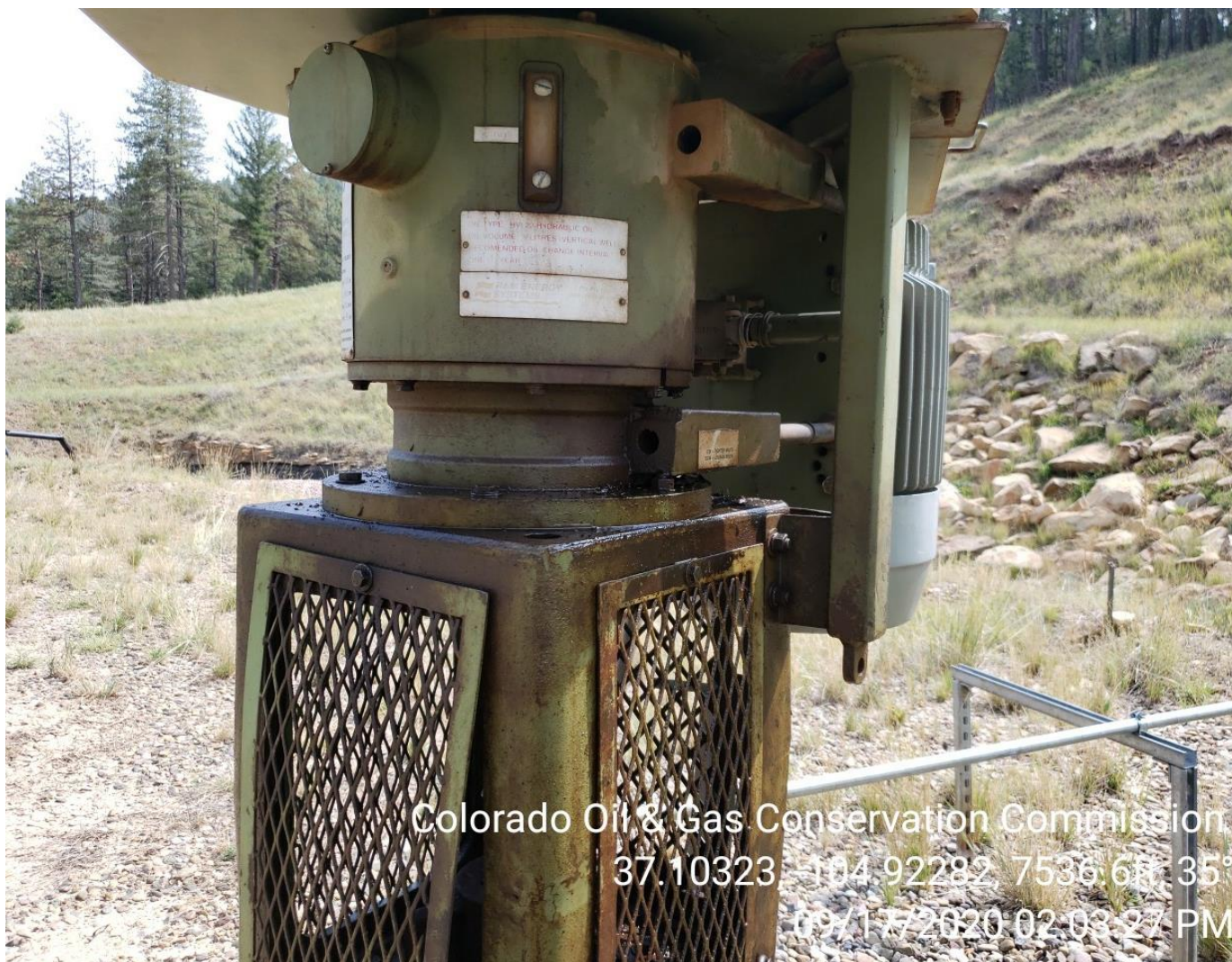
Photo 6 : Seals are leaking on drive head
