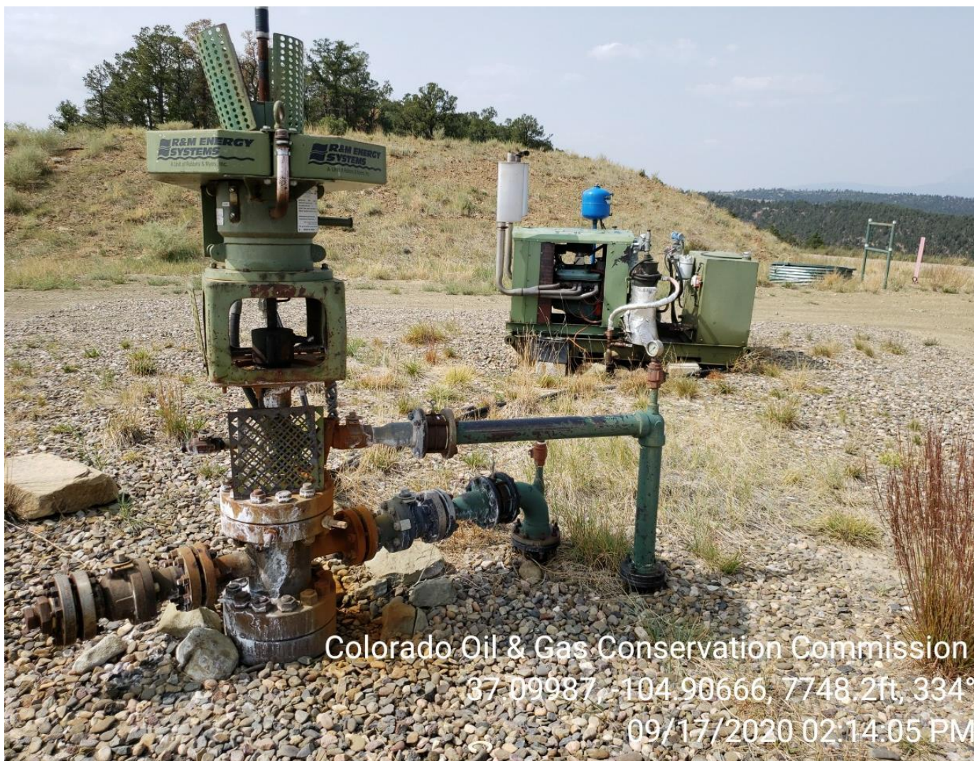
Photo 3 : Wellhead / Engine Skid
