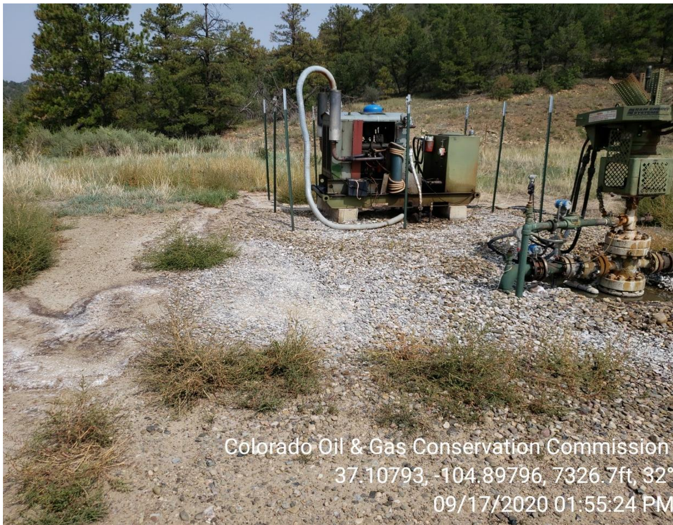
Photo 4: Stained soil from packing leak.
