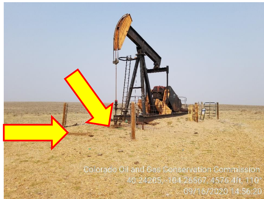
Photo 2 – Pumping Unit, Stained Soil at Wellhead
