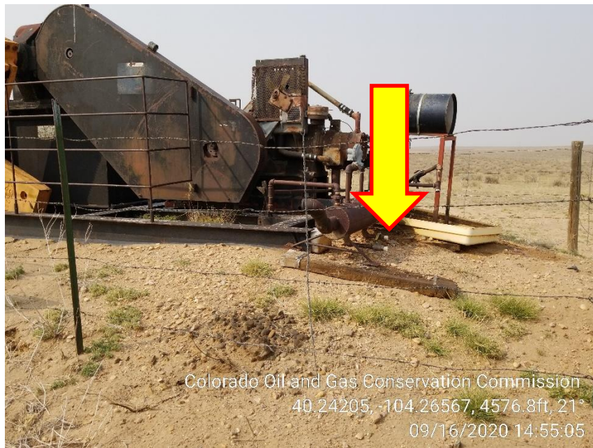
Photo 3 – Stained Soil at Gas Engine
