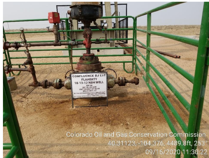
Photo 4 – 18-13-12 Wellhead Sign, Stained Soil
