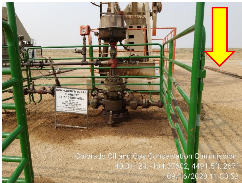
Photo 5 – 18-7-10 – Stained Soil and Unused Tubing and Rods
