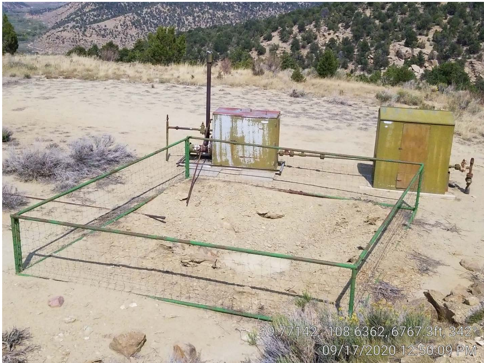
Photo 3. Separator pit, separator, meter building.
