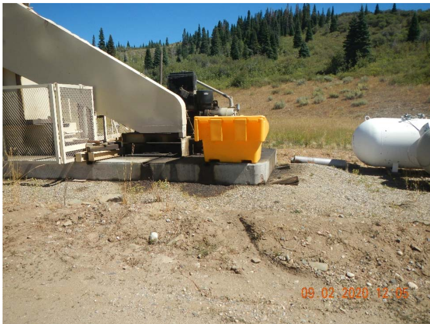
Photo 5. Stained soil at pump jack motor.
