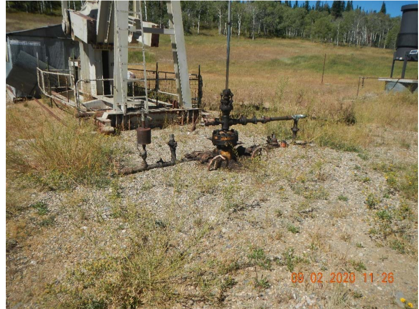
Photo 2. Stained soil at wellhead.
