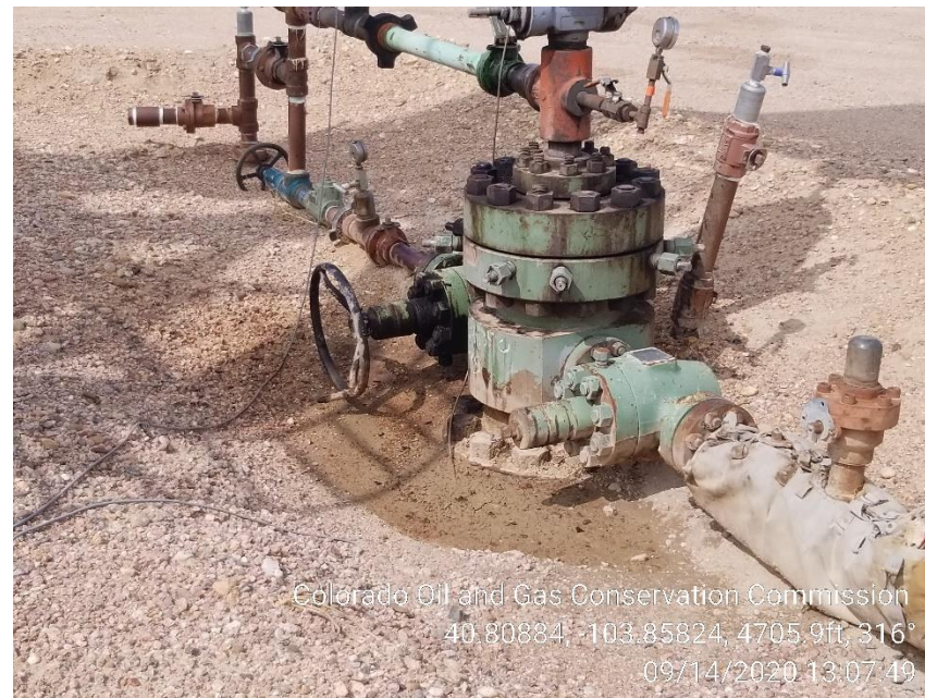
Photo 4 – 3403B Wellhead, Stained Soil
