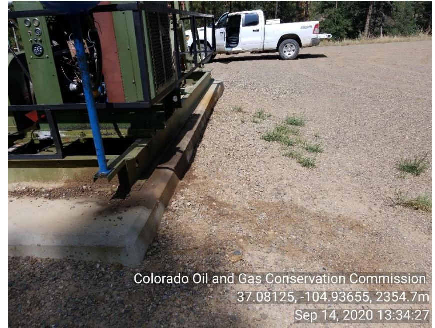
Photo 12 PU HYD leaking fluid. Stained soil and mechanical issues.
