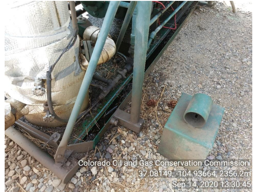
Photo 10 Stained soil around liquid ring. Mechanical issues liquid ring leaking fluid.
