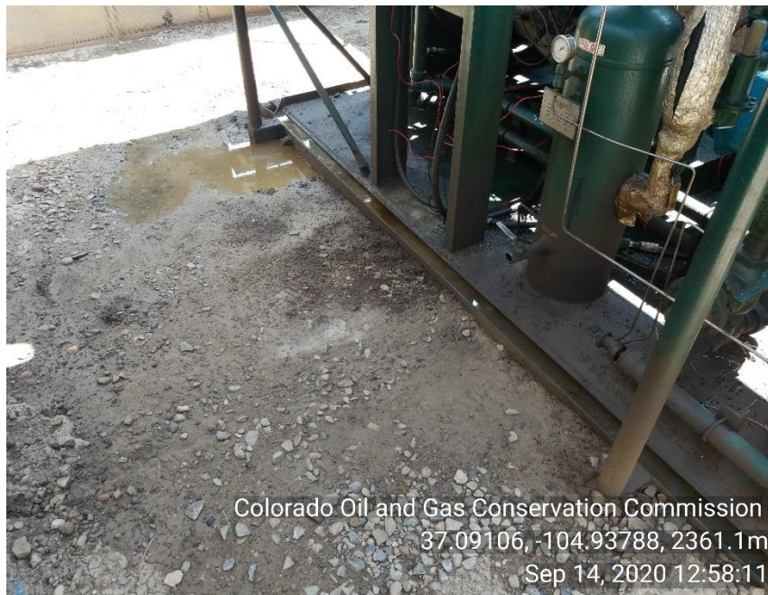
Photo 3 stained soil around liquid ring
