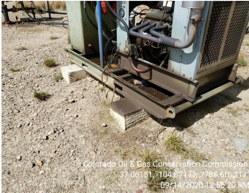
Photo 5 Stained soil at engine skid
