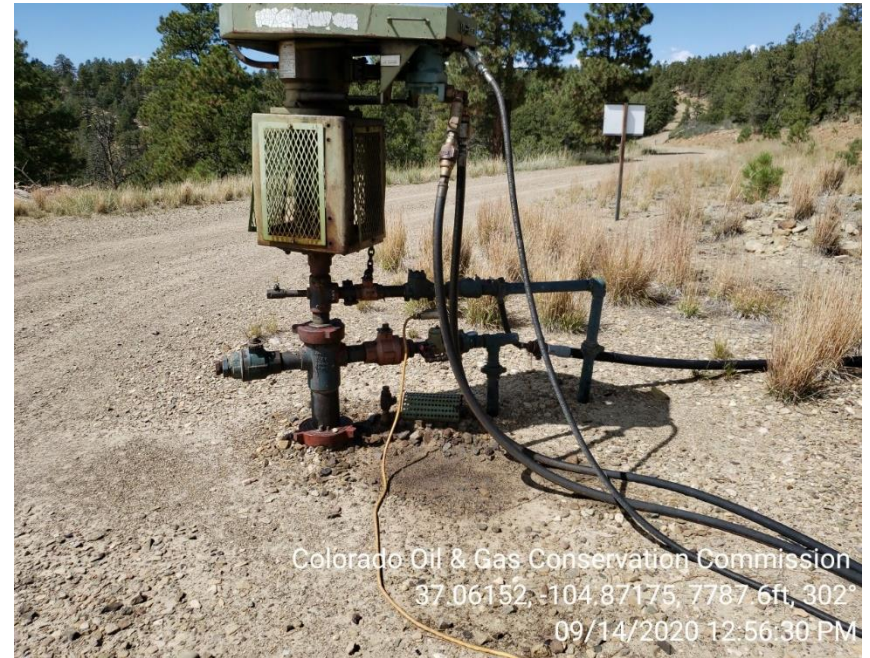
Photo 6 Stained soil at Wellhead
