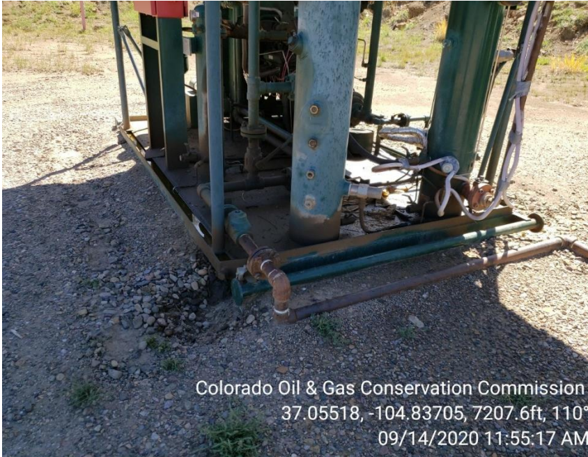
Photo 5 Stained soil at liquid ring
