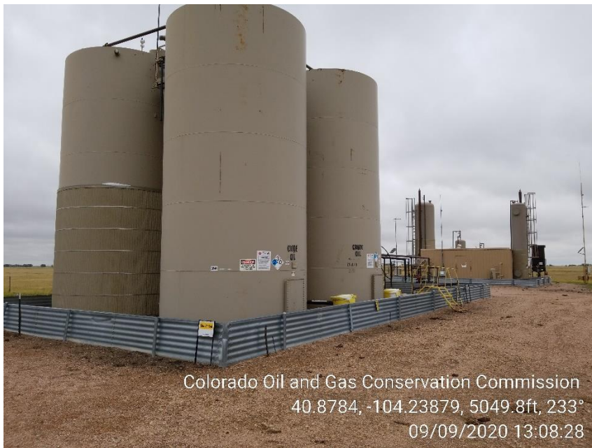
Photo 1 – Tank Battery
