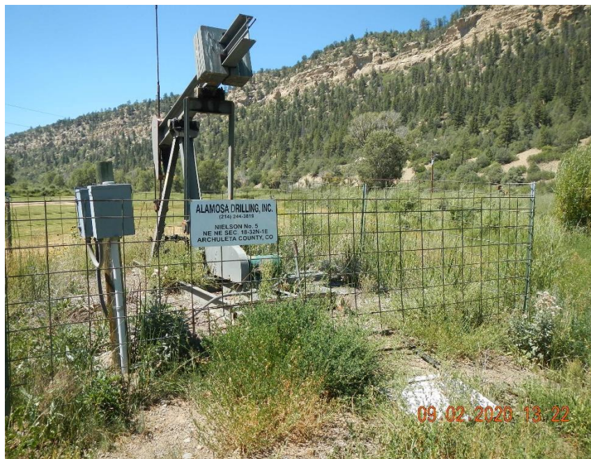
Nielson #5 well head and pump jack. Old sign remains on location.
