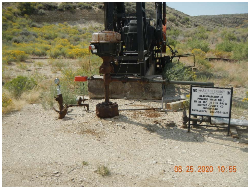
Photo 2. Stained soil at wellhead.
