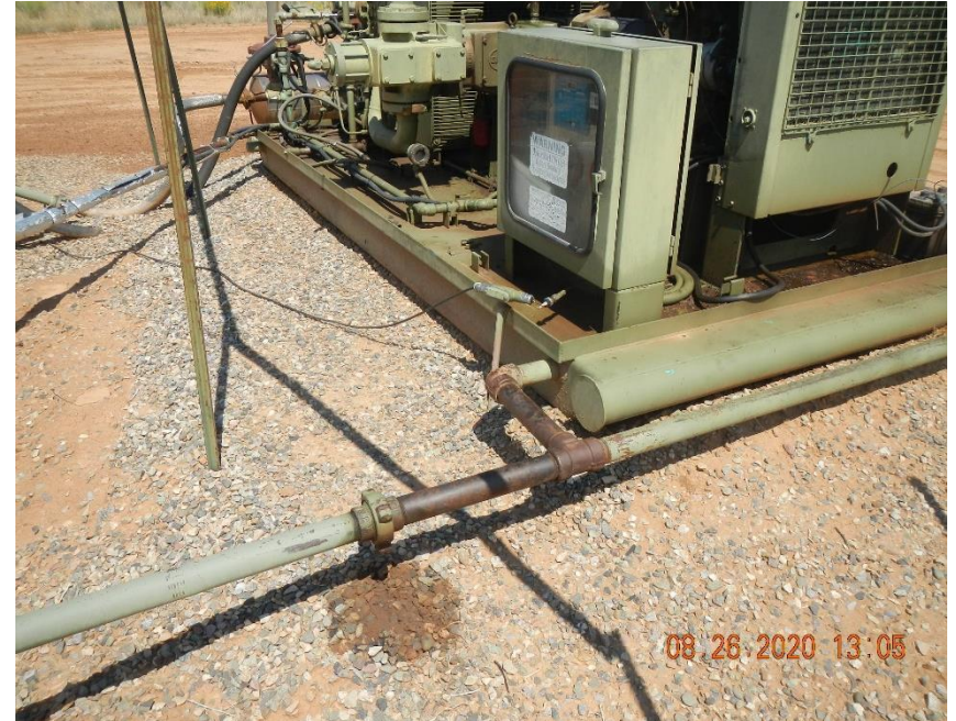
Stained soil beneath hammer union.
