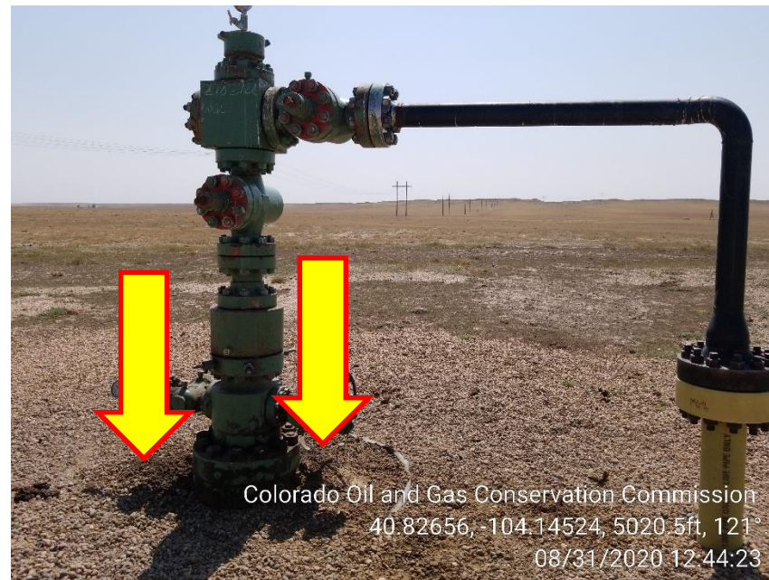
Photo 2 – Wellhead, Stained Soil
