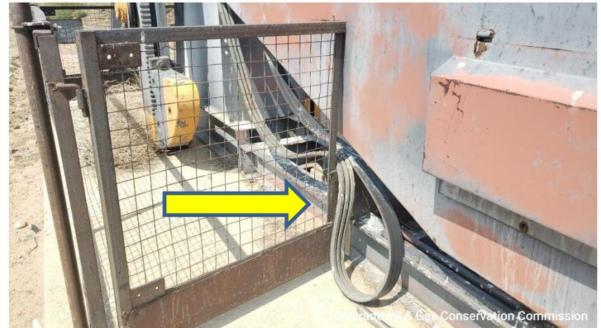
**Photo 4 unused equipment, Pump Jack belts free no motor**
