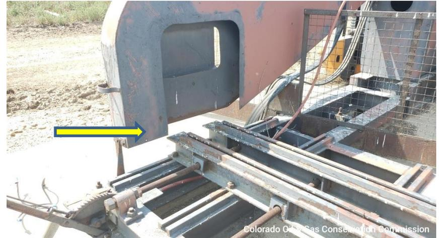
**Photo 6 unused equipment, Pump Jack has no electric motor attached to it.**
