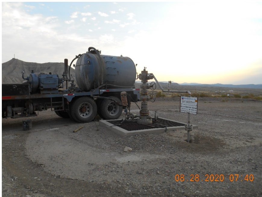
Injection wellhead
