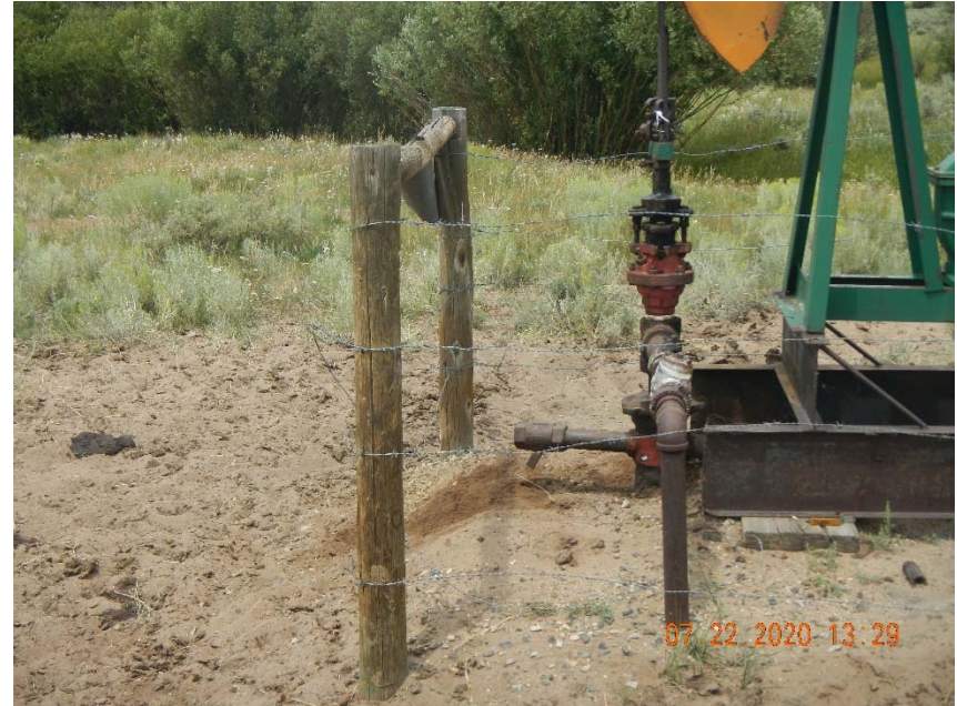
Photo 2. Stained soil at wellhead.
