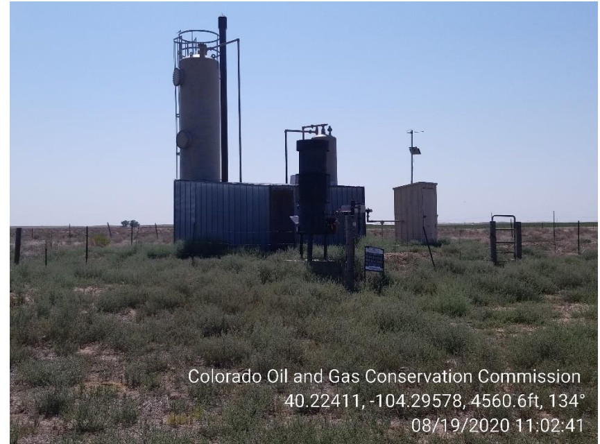
Photo 2 – Heater Treater, weeds
