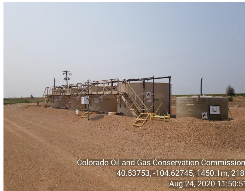
Photo 2: Tank Battery
