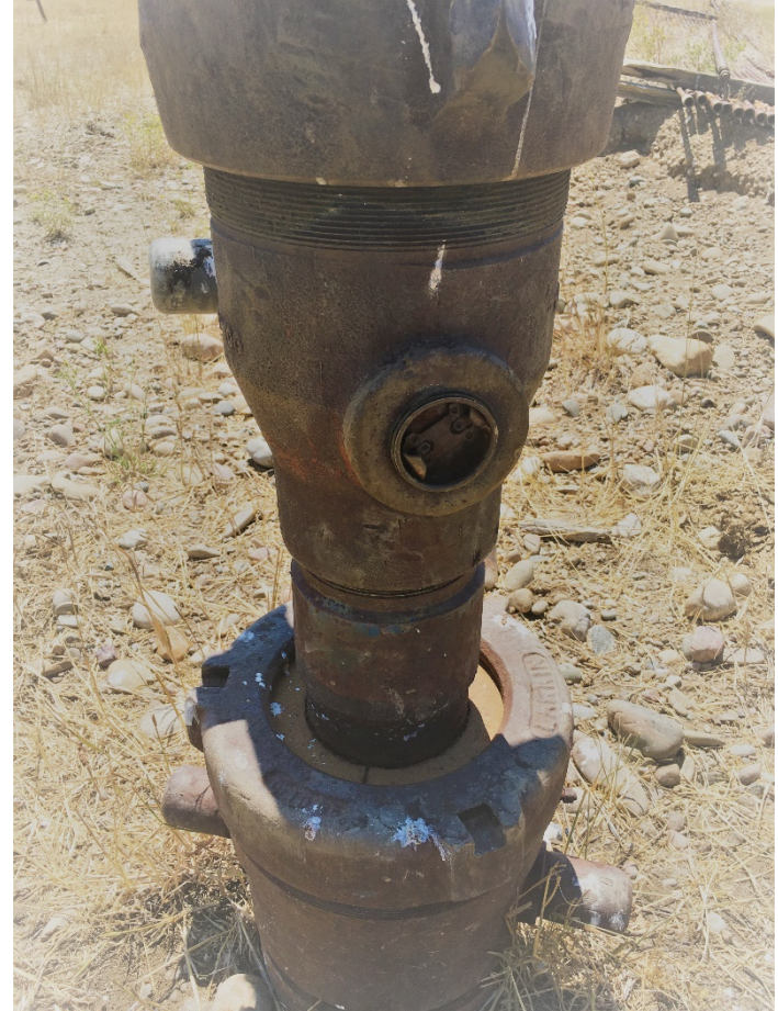
Wellhead with 55gal drum bung installed
