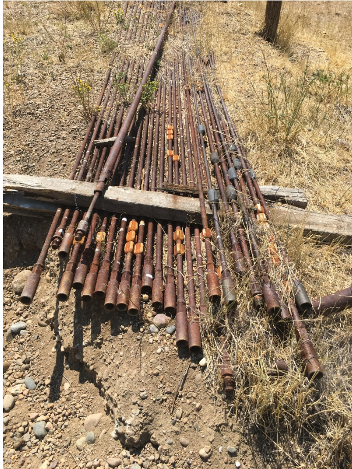
Pump and sucker rods staged by wellhead
