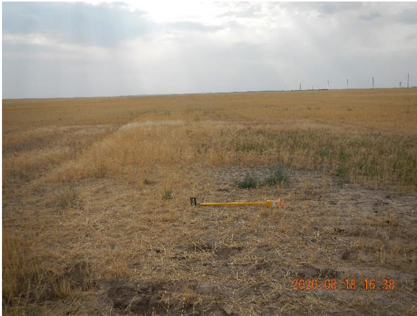
Photo 1: Locating equipment over located plugged and abandoned surface casing. Note thinner vegetation growth at plugged well site.
