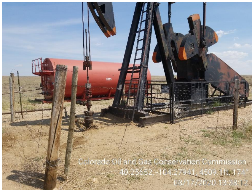
Photo 3 – Stained Soil at Wellhead, Weeds
