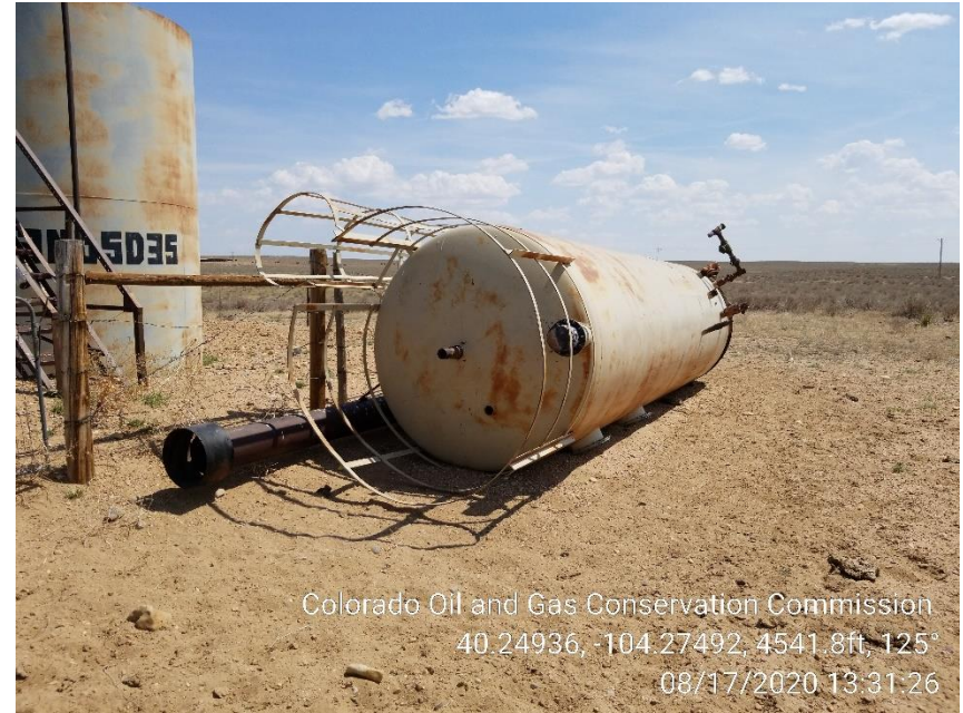
Photo 2 – Unused Heater Treater
