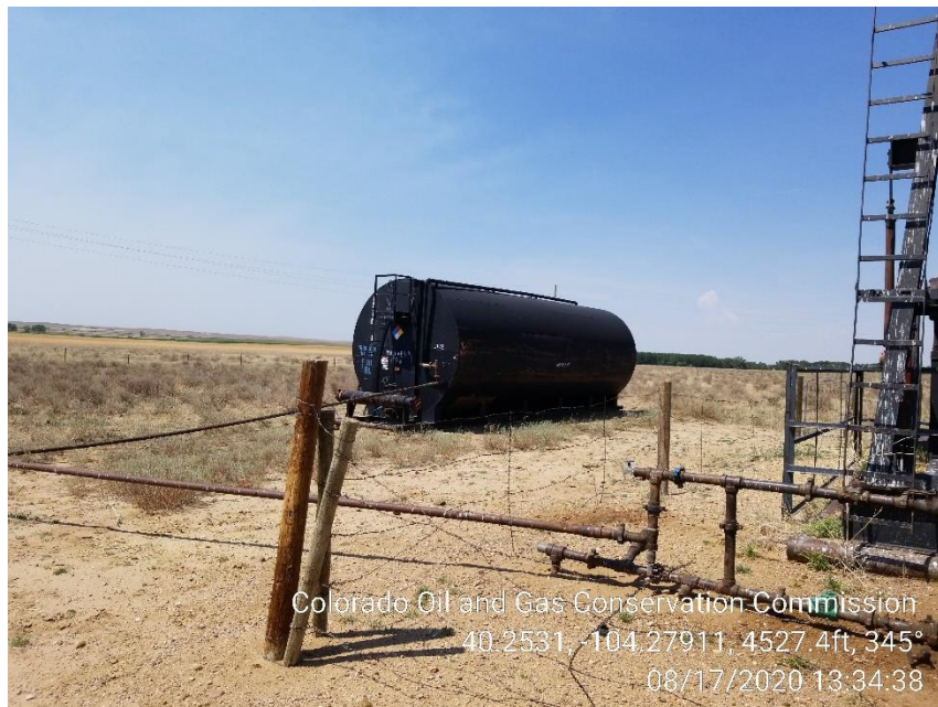
Photo 3 – Temp Tank connected to the Wellhead
