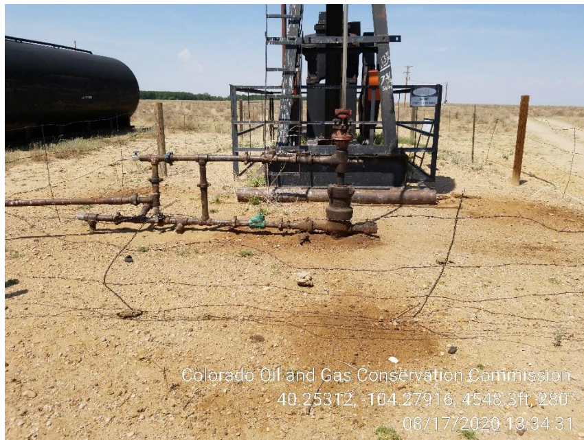
Photo 1 – Pumping Unit, Stained Soil
